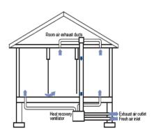
between the exhaust air and incoming air. This provides additional savings in the summer by reducing the moisture content of the incoming air that would otherwise have to be dehumidified with the cooling equipment or a dehumidifier. ERVs also provide additional comfort in the winter by adding moisture from the outgoing air to the incoming air to help avoid excessively dry indoor conditions.
